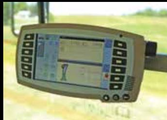
The standard Setup and Information Screen (SIS) provides quick, clear and easy analysis of operating data. With one glance, you can check basic information on tractor
